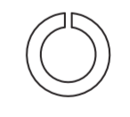
eight \Phi 8 Spring Washer (#91)
